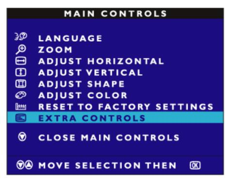
3) Press the MENU button. The EXTRA CONTROLS window appears. ADJUST MOIRE will be highlighted.
